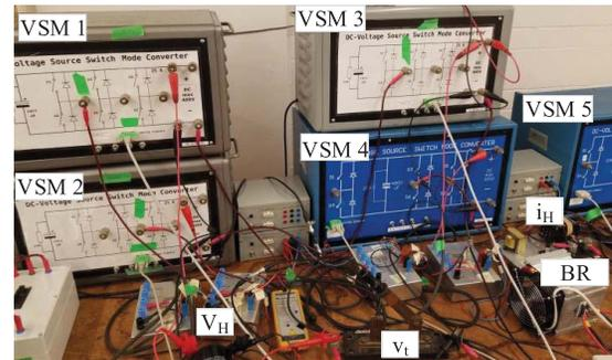
Fig. 8. Experimental setup. BR denotes the bridge rectifier.
