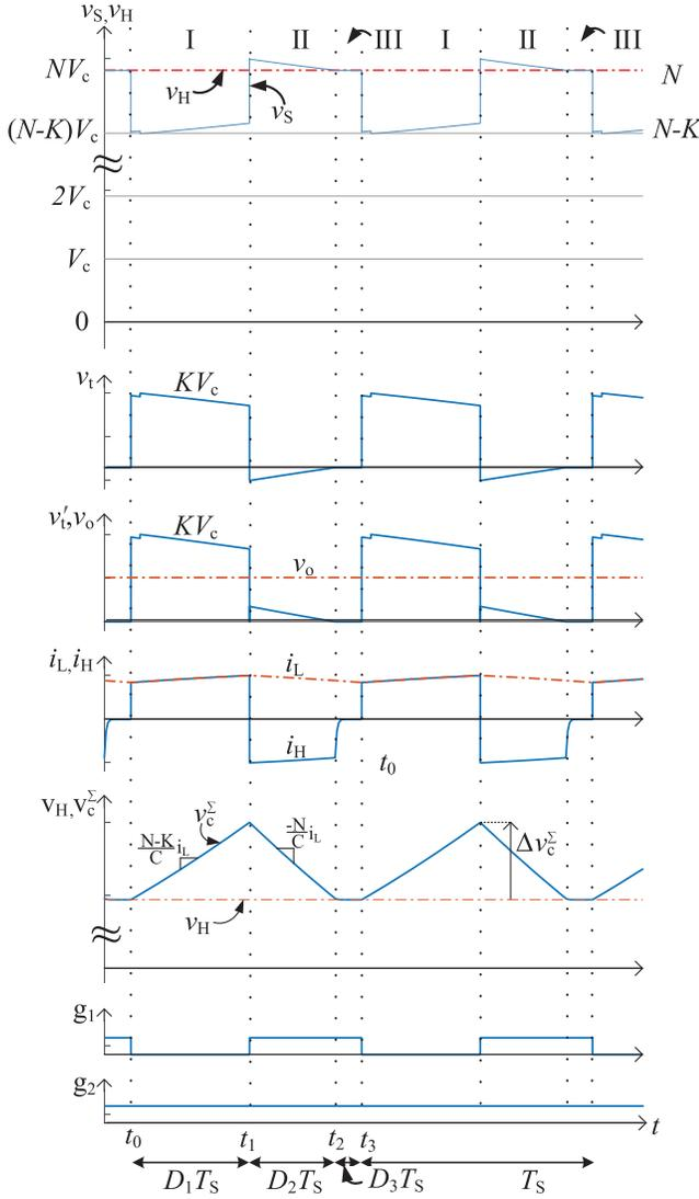
Fig. 4. Representative steady-state operating waveforms. Intervals I–III correspond to the charge, discharge, and freewheeling operating modes, respectively. The number of switched cells  $K = 1$ . The number of cells  $N = 4$ .
