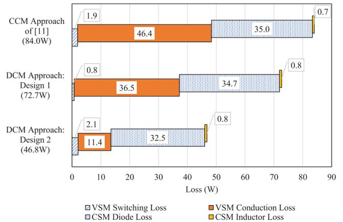
Fig. 12. Loss comparison. Total losses for CCM approach, DCM Design 1, and DCM Design 2. The simulated operating point is 3750–380 V with 5.7 kW of power and a fundamental ac frequency of 5 kHz.
