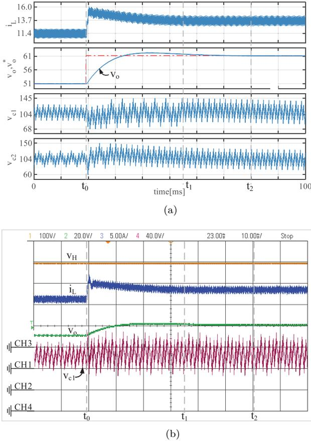
Fig. 11. Experimental transient results: 20% step change in output voltage reference  $V_o^*$  from 51 to 61 V<sub>dc</sub>. (a) Simulation results for validation. (b) Experimental results. CH1 =  $v_H$ , CH2 =  $v_o$ , CH3 =  $i_L$ , and CH4 =  $v_{c1}$ .
