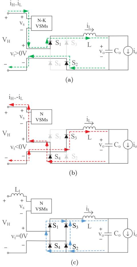
Fig. 3. Operating modes. (a) Charge mode:  $v_t > 0$  and  $i_H = i_L$ . Total duration is  $D_1 T_s$ . (b) Discharge mode:  $v_t < 0$  and  $i_H = -i_L$ . Total duration is  $D_2 T_s$ . (c) Freewheeling mode:  $v_t = 0$  and  $i_H = 0$ . Total duration is  $(1 - D_1 - D_2) T_s$ .
