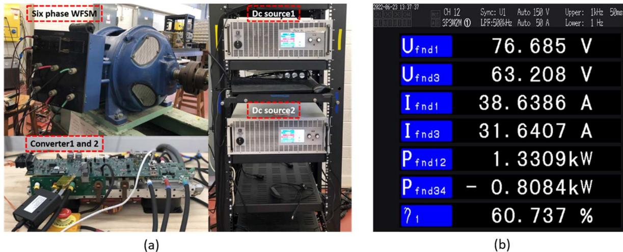
Fig 8: (a) Experimental setup (six-phase WFSM, dual inverter system, and two DC sources) (b) power analyzer results: machine line voltages, currents, power, and efficiency.
